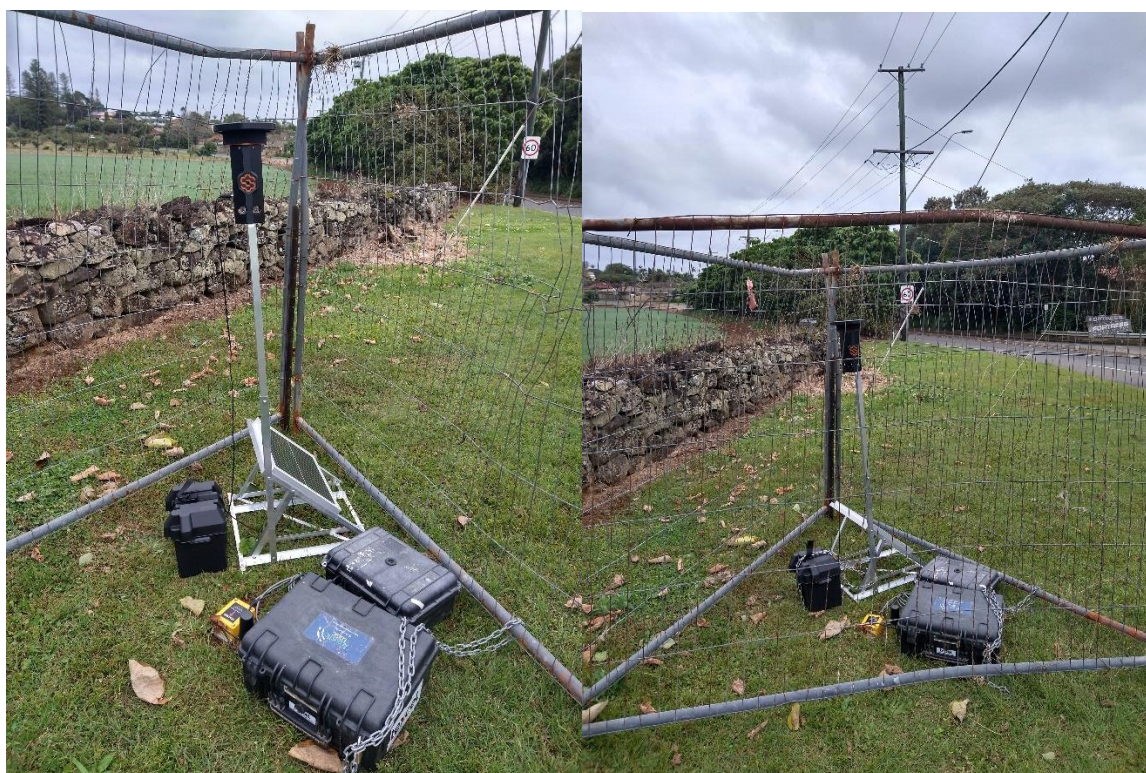
Figure 3-1 Noise, Dust and Vibration Monitor Installation Locations
